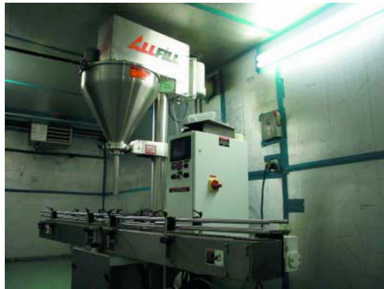
Powder fill unit, that dispenses BarleyMax®, CarrotJuiceMax™ and BeetMax, into our plastic containers.
